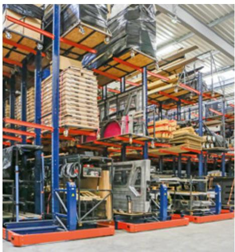
SI POSSONO COLLOCARE SU BASI MOBILI PER AUMENTARE LA CAPACITÀ DI STOCCAGGIO.
