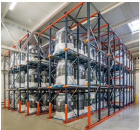
FUNZIONANO CON IL SISTEMA LIFO (*LAST IN, FIRST OUT*)
