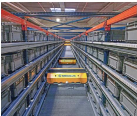
SI ADATTA ALLE DIFFERENTI UNITÀ DI CARICO: CASSE IN PLASTICA, CARTONE O VASSOI METALLICI DI DIFFERENTI MISURE.
